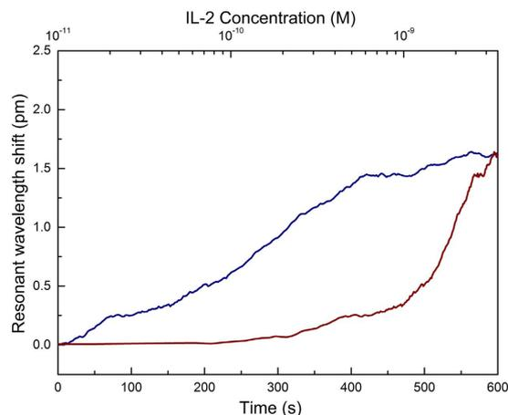
**Figure 5. Sensitivity of the microtoroid biosensor.** Human IL-2 protein in 1 $\times$  PBS buffer was used as an analyte for  $\alpha$ -IL 2 antibodies. The infusion started at  $t=0$  and continued for 600 s with an infusion rate of 5  $\mu\text{l/s}$ . The blue line represents the shift with respect to time, while the red line is the response in terms of WGM resonance shift with respect to IL-2 concentration.
