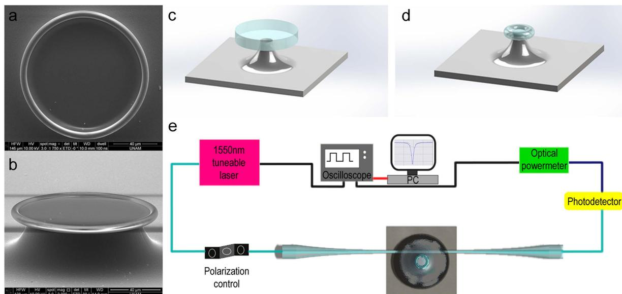
**Figure 2. Microtoroid fabrication and optical coupling setup.** Microtoroids (a,b) were fabricated by reflow of microdisks following microfabrication (c) by a CO<sub>2</sub> laser (d). The optical setup consists of a tuneable laser, a polarization controller, a powermeter and an oscilloscope. All setup could be controlled with a custom built software.
