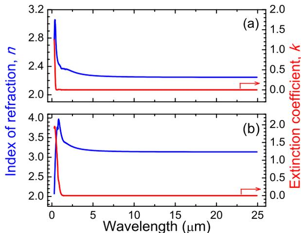
FIG. 2. (Color online) Measured index of refraction and extinction coefficient of (a) thermally evaporated As<sub>2</sub>S<sub>3</sub> and (b) Ge<sub>15</sub>As<sub>25</sub>Se<sub>15</sub>Te<sub>45</sub> thin films. The refractive index contrast allows to achieve omnidirectional photonic band gap.
