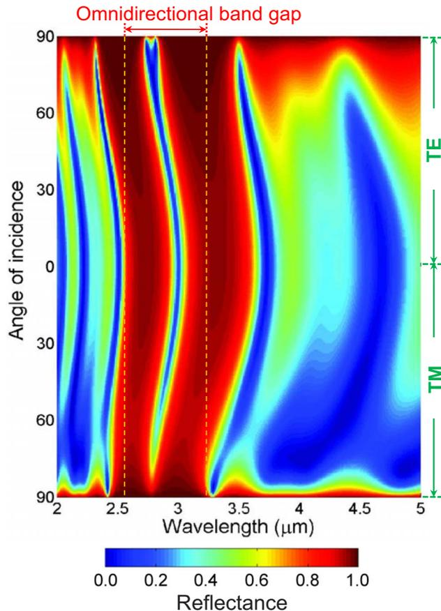
FIG. 4. (Color online) Calculated reflectance spectra of the omnidirectional filter as a function of wavelength for TM and TE polarizations for all angles of incidence at a position having the band gap centered around 3 μm.
