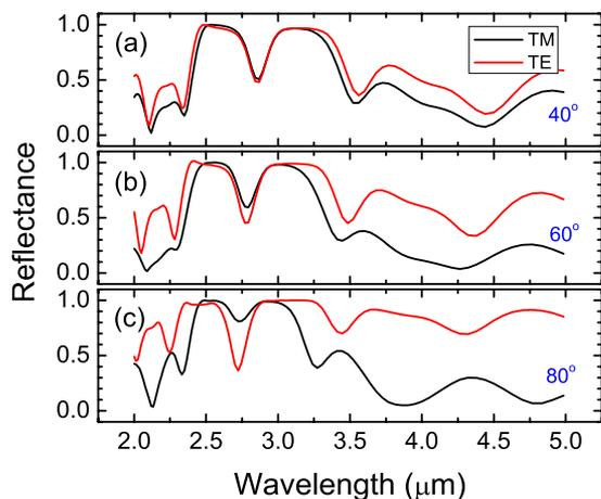
FIG. 5. (Color online) Measured reflectance spectra of the filter as a function of wavelength for (red lines) TE and (black lines) TM polarization modes at (a) 40°, (b) 60°, and (c) 80° angles of incidence.
