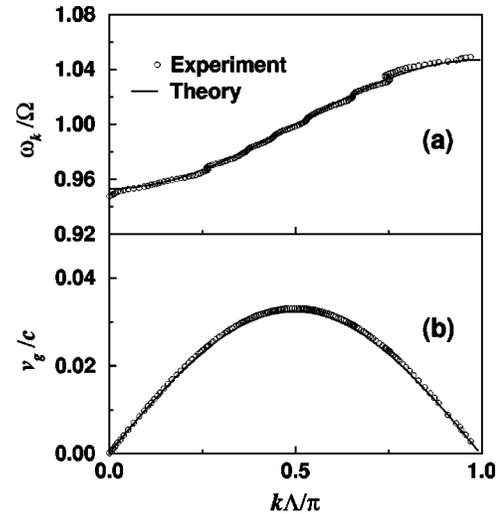
FIG. 4. (a) The dispersion relation of the waveguiding band for the zig-zag shaped CCW. Experimental curve was obtained from the transmission-phase measurements via Eq. (1). (b) Group velocity  $v_g$  as a function of wave vector  $k$ . The measurements are in good agreement with the tight-binding predictions.
