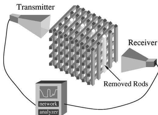
FIG. 2. Experimental setup for measuring the transmission-amplitude and transmission-phase spectra of the coupled cavity waveguides (CCW) in 3D photonic crystals.
